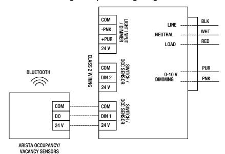
NOTE: Communications can be done through the Bluetooth Mesh network or be wired when using 24 VDC.
